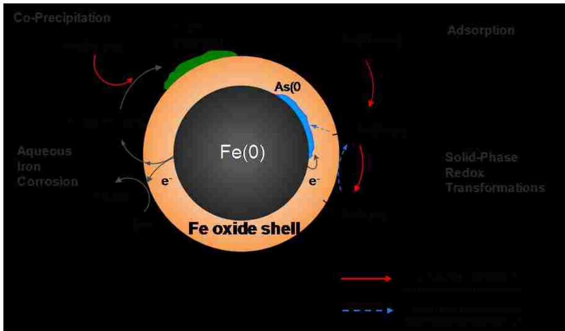
Figure 7.17 Schematic diagram summarizing processes responsible for arsenic removal in As(III)-nZVI system in anoxic conditions. The relative scale of the core and shell components of nZVI are for illustration only and do not reflect actual dimensions. As(III) may be taken up from the aqueous phase by adsorption or co-precipitation. The solid-bound As(III) is oxidized rapidly at the oxide surface, and the As(V) formed may be reverted to As(III) at a slower rate. Some As(III) diffuses towards Fe(0) core and is reduced to elemental arsenic (As(0)) near the oxide/Fe(0) interface.
